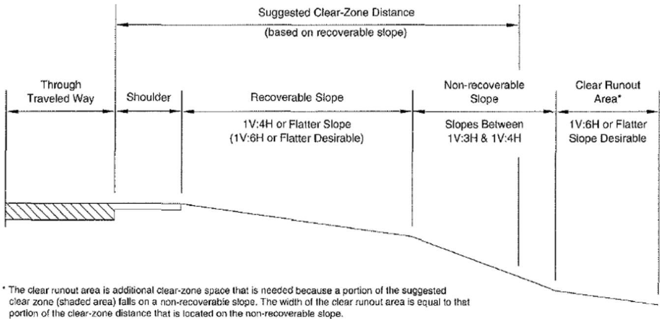
Figure 2 - Clear zone for non-recoverable parallel foreslope (Source: Roadside Design Guide).
