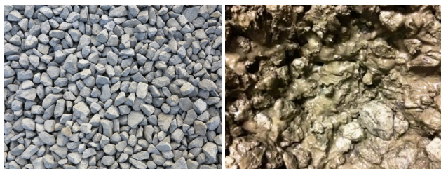
Figure 5 - Under-slab clear stone (a) without contamination (b) contaminated with fine soil particles.
