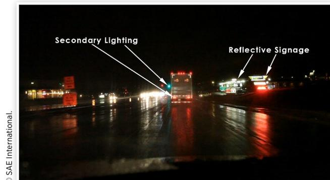
sources, and the reflection can be seen on the roadway surface. *Figure 31* is an example of secondary lighting and reflective signage on the roadway.
