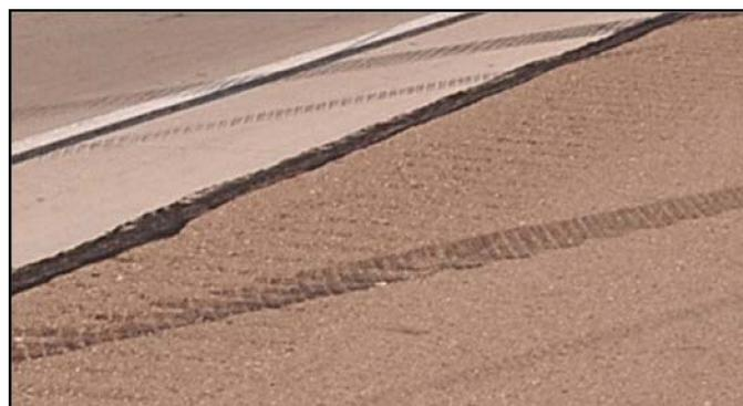
Figure 1. Striated tire marks deposited by a yawing vehicle.
