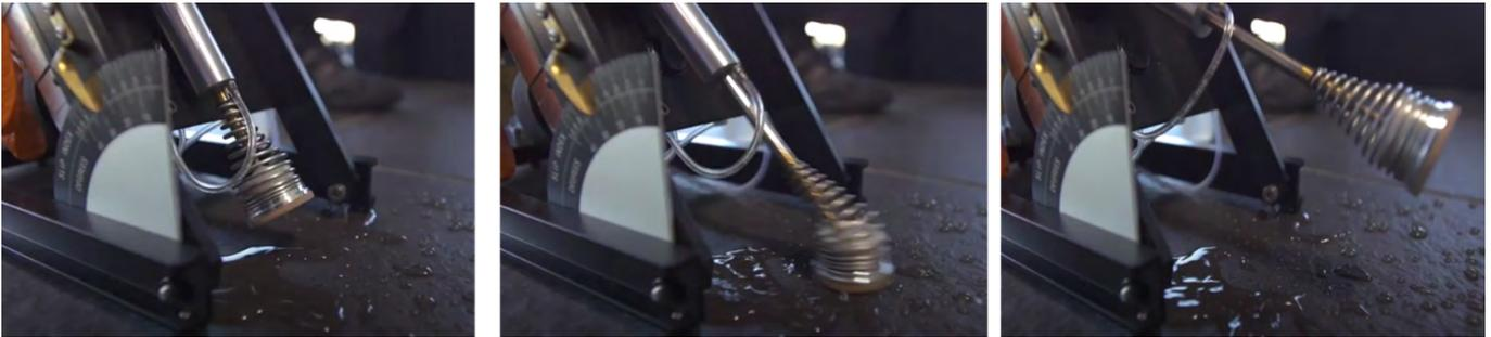
**Figure 1** - Excel tribometer testing wet surface
