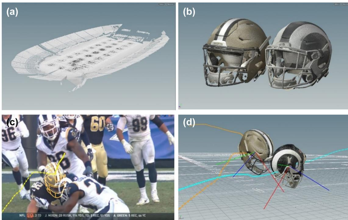
**FIGURE 1.** Three-dimensional scans of the stadium (a) and player helmets (b) that were used for the videogrammetry calibration process. (c) Three-dimensional helmet scan overlaid in the video frame that was used to track helmet position and orientation with respect to the field throughout the impact time history (d).
