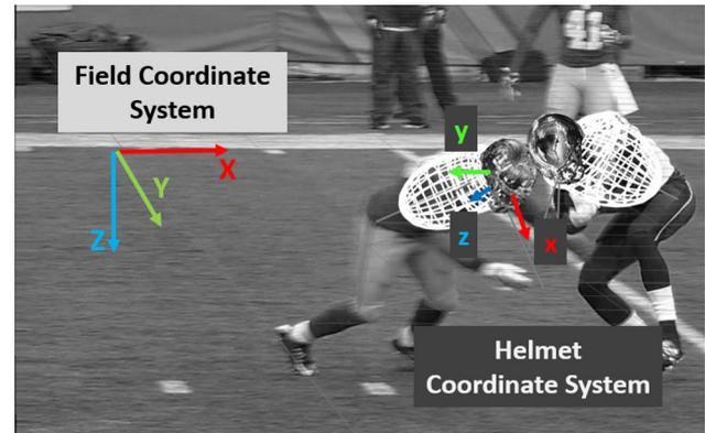
**FIGURE 2.** Helmet and field coordinate systems used for video reconstruction data processing. Lower-case subscripts denote a local coordinate system while the upper-case subscripts denote the global (inertial) coordinate system. Ellipsoids for quantifying torso orientation are also shown.
