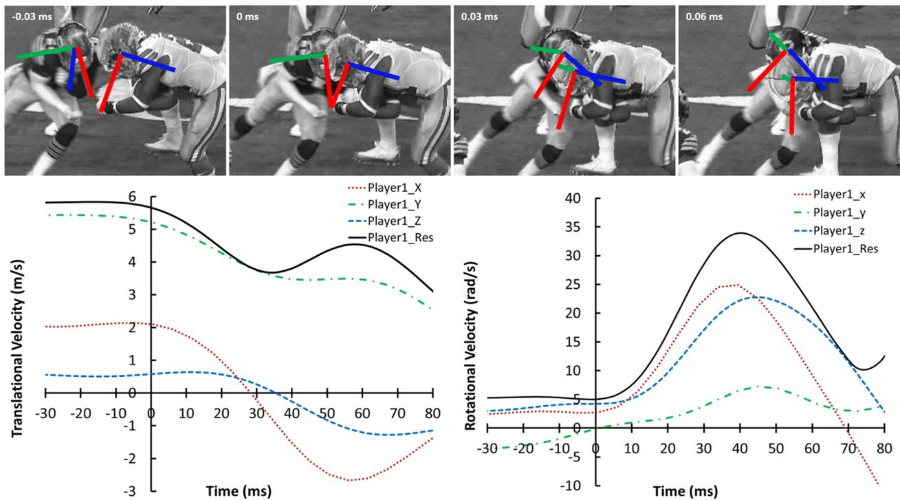
**FIGURE 3.** Sample translational (field coordinate system) and rotational (helmet coordinate system) velocity time-histories for Player1 for Case 06 helmet-to-helmet impact, where  $t = 0$  is  $t_0$ . Snapshots from the video with overlaid 3D images of the helmets are provided, with Player1 on the left, and Player2 on the right.
