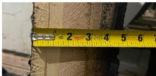
Figure 10 - Charred CLT surface (top) and uncharred layer of CLT panel (bottom) after fire exposure.
