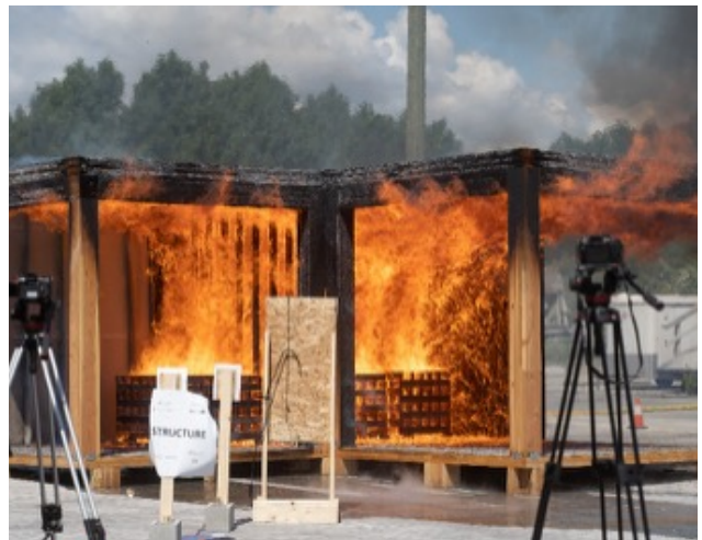
Figure 9 - Large-scale compartment fire test of CLT construction.
