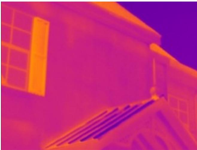
**Figure 8** - Low contrast thermal image with wide temperature span
