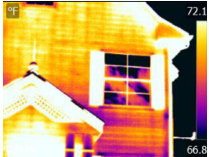
*Figure 2 - Thermal anomalies at bottom left corner of window*
