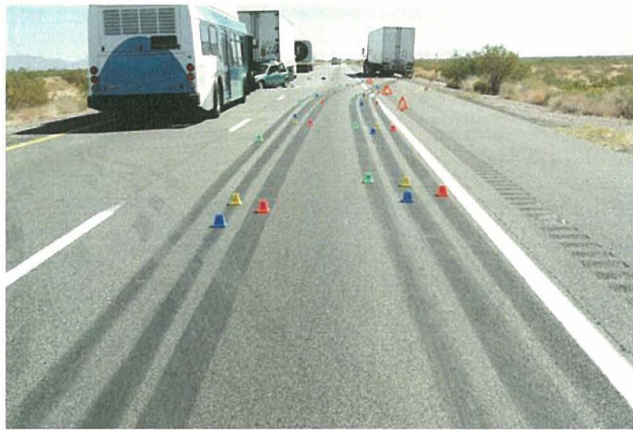
Figure 8. Tire marks due to trailer swing from accident (left) and testing (right).
