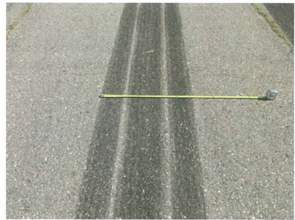
Figure 8. Tire marks due to trailer swing from accident (left) and testing (right).
