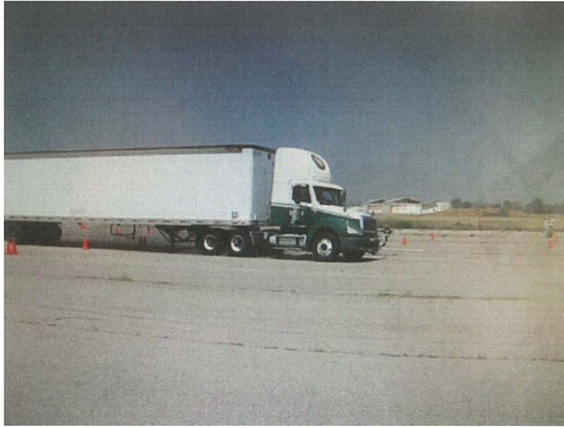
Figure 10. Tractor wheel lift during lane change.
