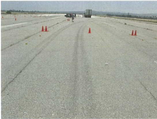
Figure 5. Braking marks with trailer ABS on.
