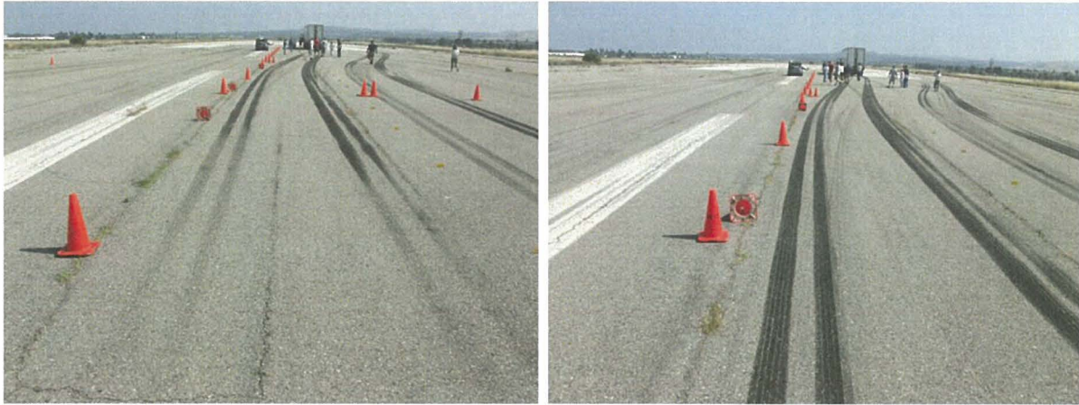
Figure 7. Tire marks from trailer with ABS disabled.
