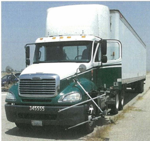
Figure 4. Test cameras mounted on tractor and chase vehicle.
