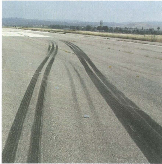
Figure 6. Tire marks from first test with ABS disabled.
