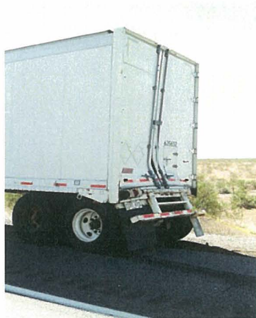
Figure 3. Damage to rear of trailer due to undercarriage motion.
