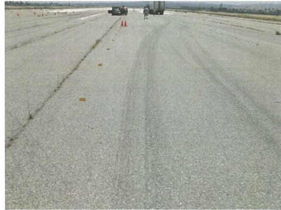
Figure 5. Braking marks with trailer ABS on.
