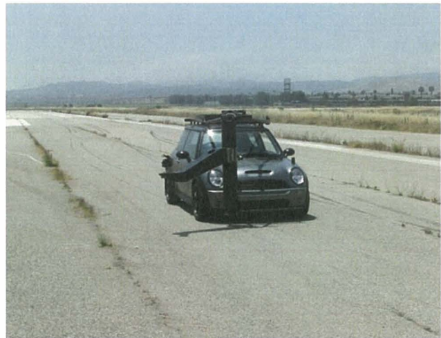
Figure 4. Test cameras mounted on tractor and chase vehicle.
