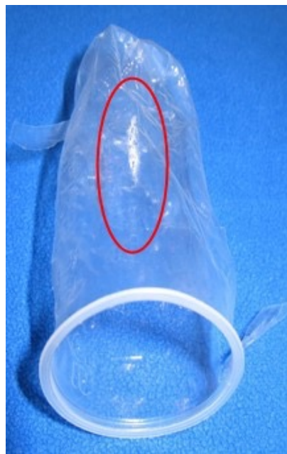
Figure 1 - Wax-like contamination on the surface of polyethylene plastic baby bottle liners.
