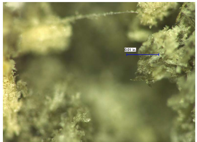
Figure 19 - Scrapings from needle valve housing (bore), 200X magnification.
