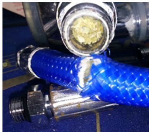
Figure 11 - Severely degraded TPU hose clogging air hose.
