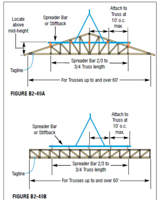
Figure 5 - Example of how spreader bars are used for truss hoisting (Source: BCSI Canada).
