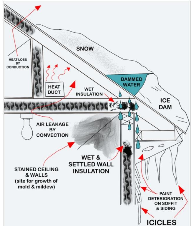
Figure 9- Schematic of ice damming (Source: <https://extension.umn.edu/protecting-home-rain-and-ice/dealing-and-preventing-ice-dams>).
