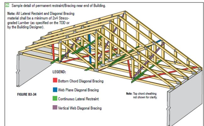
**Figure 3** - Typical permanent truss system bracing (Source: BCSI Canada).
