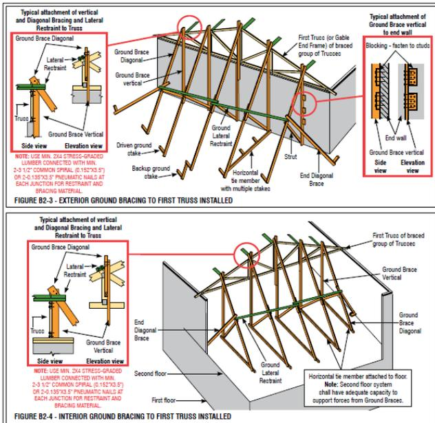
Figure 4 - Example of gable truss bracing during truss installation (Source: BCSI Canada).
