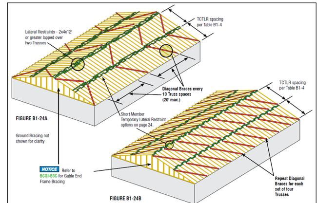
**Figure 2** - Typical temporary top chord bracing for erection (Source: BCSI Canada<sup>1</sup>)
