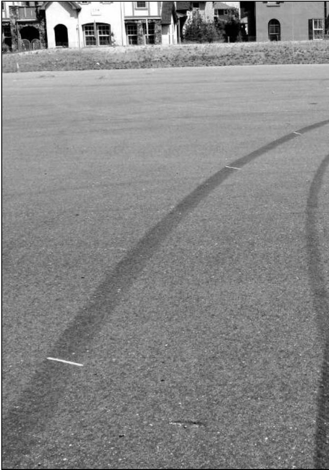
**Figure 16** - Left rear tire mark from Test 2.
