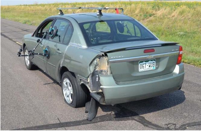
Figure 4. Photograph of Axle Wrap Test at Rest.
