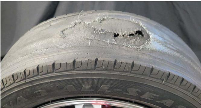
Figure 5. Photograph of the Test Tire that Experienced Lockup.
