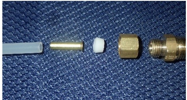
Exploded compression connection components
