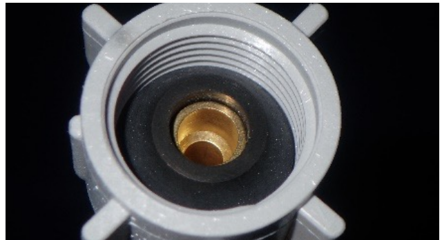
Compression fitting with polymer gasket
