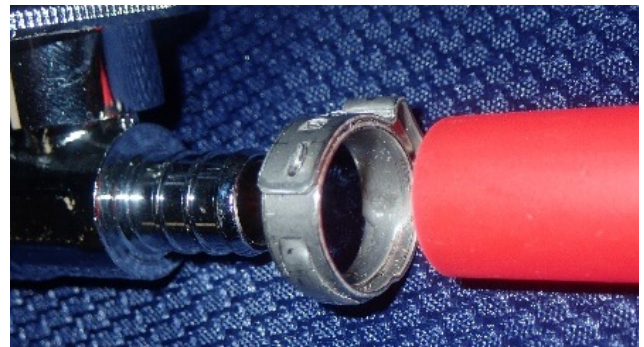
Exploded view of pinch clamp connection
