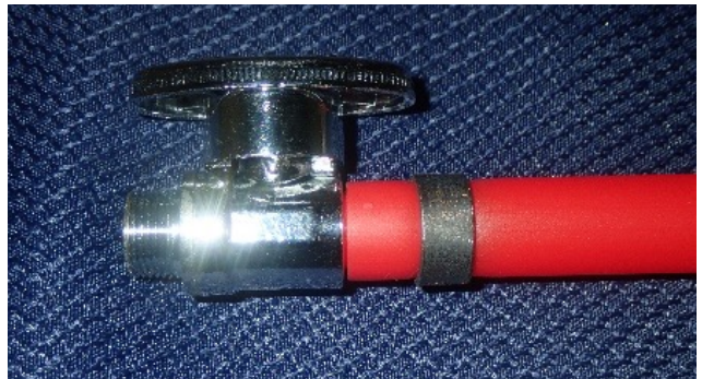
Crimp ring positioned too far from fitting
