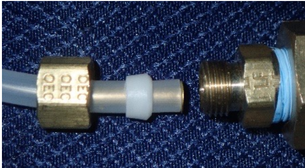
Incorrect ferrule orientation
