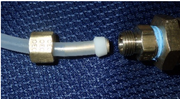
Insufficient tube insertion
