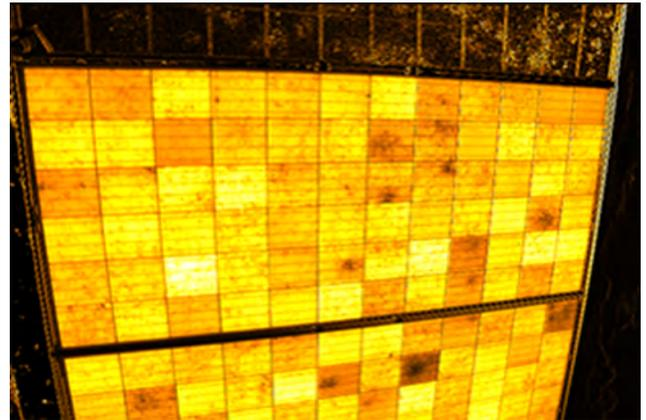
*Figure 4 - Electroluminescence testing on solar panels.*
