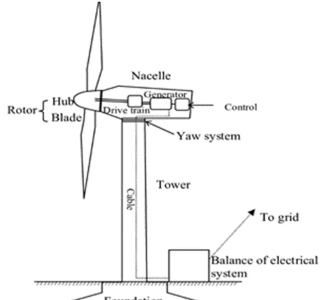
**Figure 2** - Basic layout of a typical wind turbine's major components.
