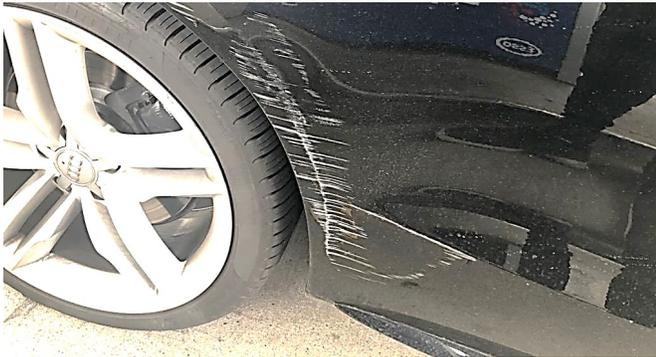
**Figure 2** - Views of the sharp scratches that result from contact with a stationary object such as a wall/pole.
