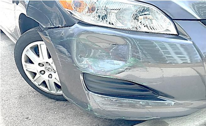
**Figure 1** - View of the excessive paint transfers that result from contact with a painted stationary object such as a wall/pole.
