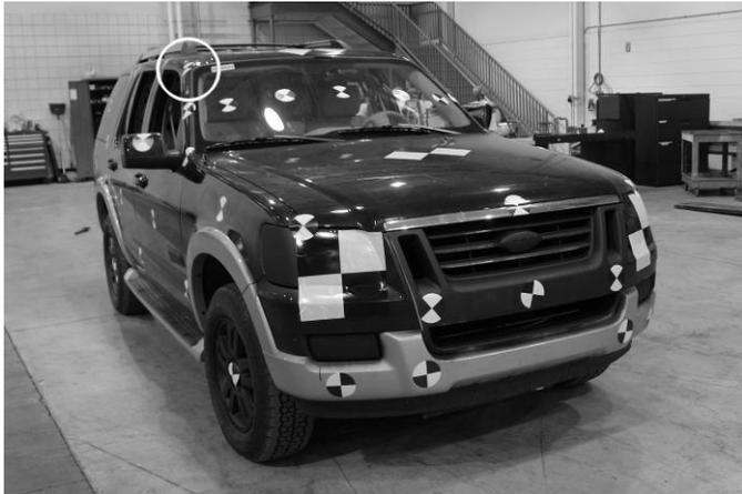
**Figure 21 – Fiducial Sticker on Passenger’s Side A-Pillar Used for Deformation Measurement**
