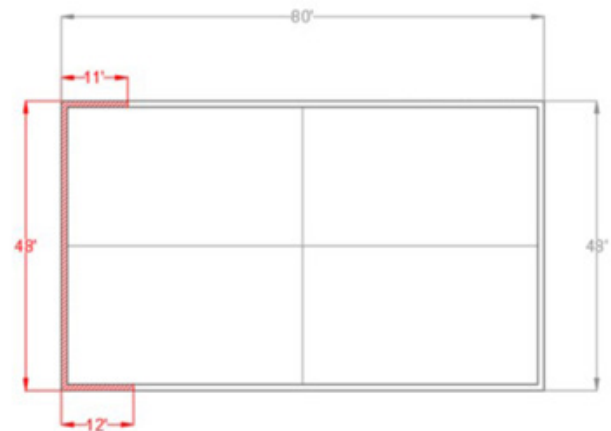
Figure 1 - Plan view of a building with areas of collapsed wall denoted in red.
