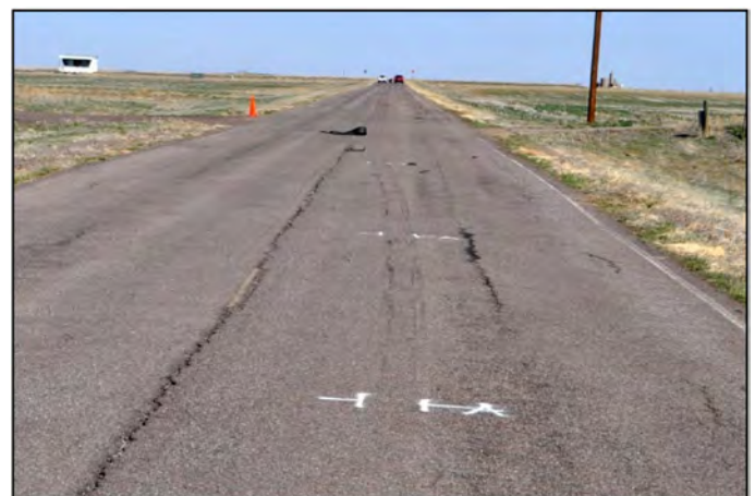
Figure 17. Tire mark from a full tread separation with air loss
