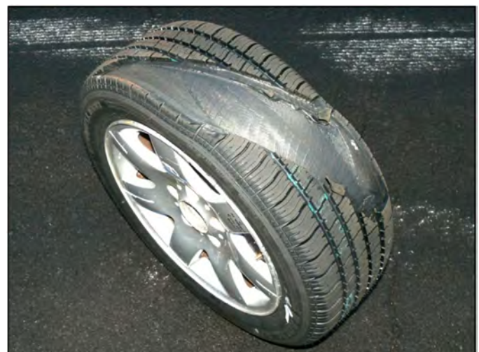
Figure 30. Tire following a partial separation in the trailing direction
