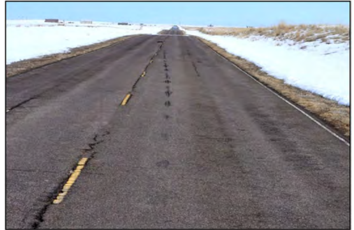
Figure 15. Tire mark from a full tread separation test
