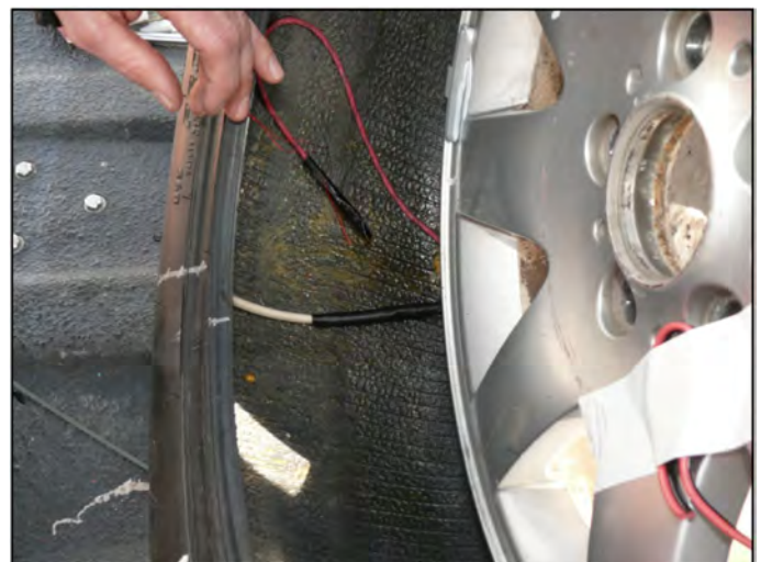
Figure 12. Detonation cord on the interior of the tire
