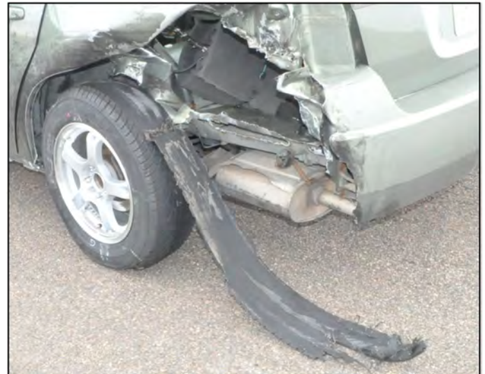
Figure 24. Tire following a partial tread separation test where the tread flap remained attached
