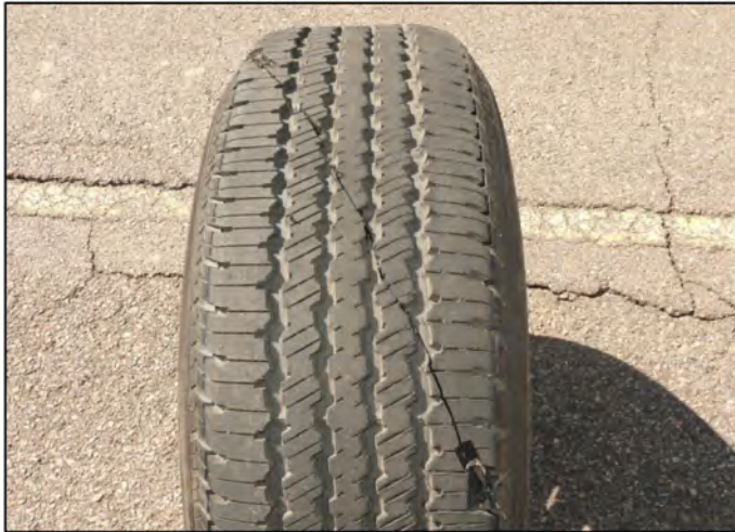
Figure 8. Example of bias cut across tread
