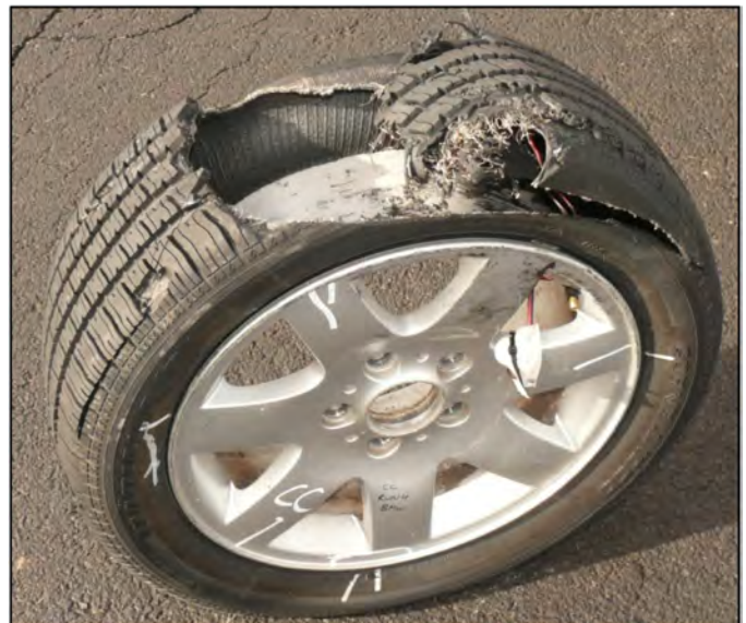
Figure 29. Tire following a blowout
