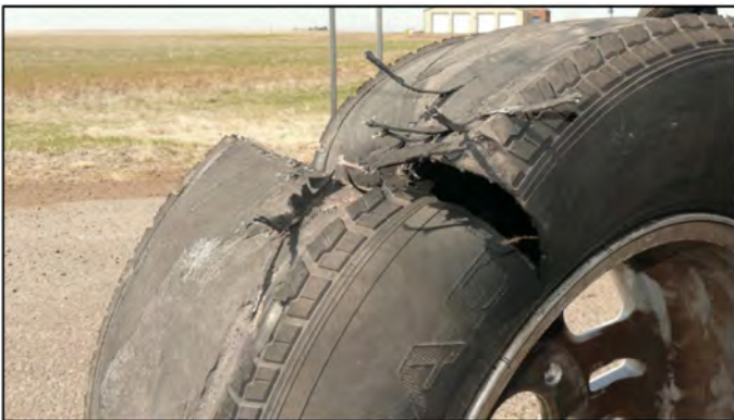
Figure 27. Tire following a full tread separation with unintended air loss
