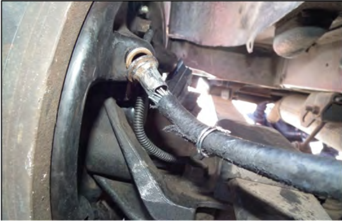
Figure 22. Damage to parking brake cable following test C04
