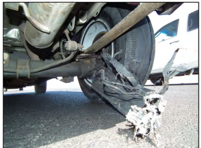
Figure 21. Tread lodged following test C04
