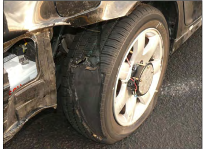
Figure 28. Tire following a trailing partial separation with air loss
