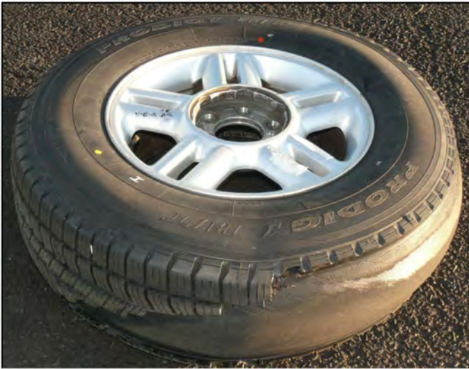
Figure 26. The tire following a partial tread separation test where the tread flap detached leaving 180 degrees of tread remaining on the tire
