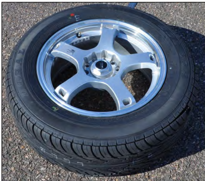
Figure 9. Example circumferential shoulder cut
