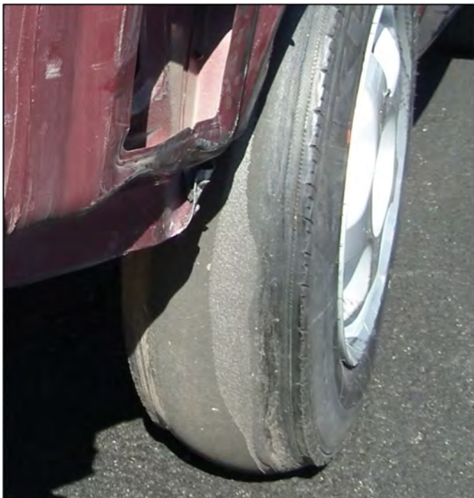
Figure 23. Tire following a full tread separation test
